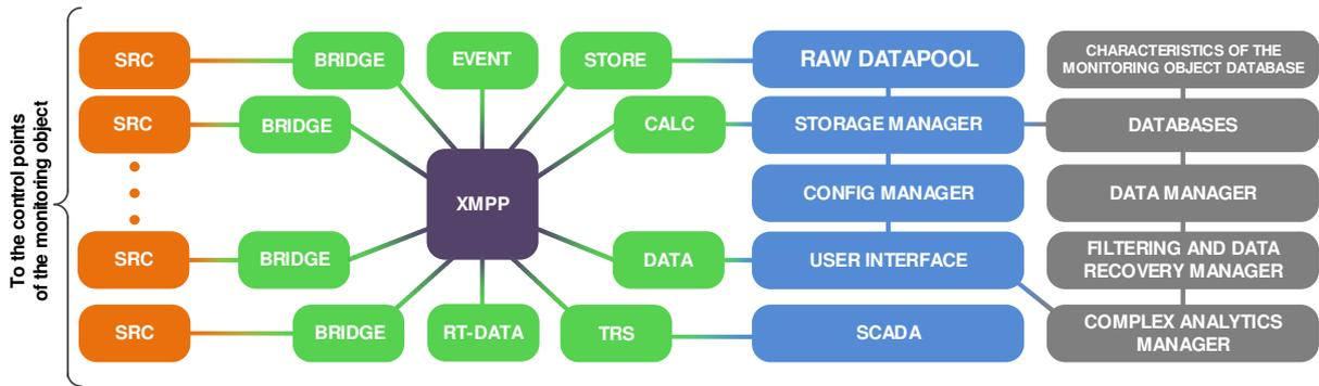
Figure 2. Architecture of a universal monitoring system
